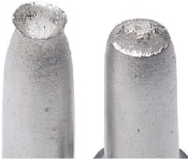
cup-and-cone fracture - moderately ductile
