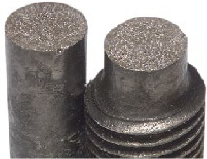
brittle fracture - totally brittle - flat surfaces
